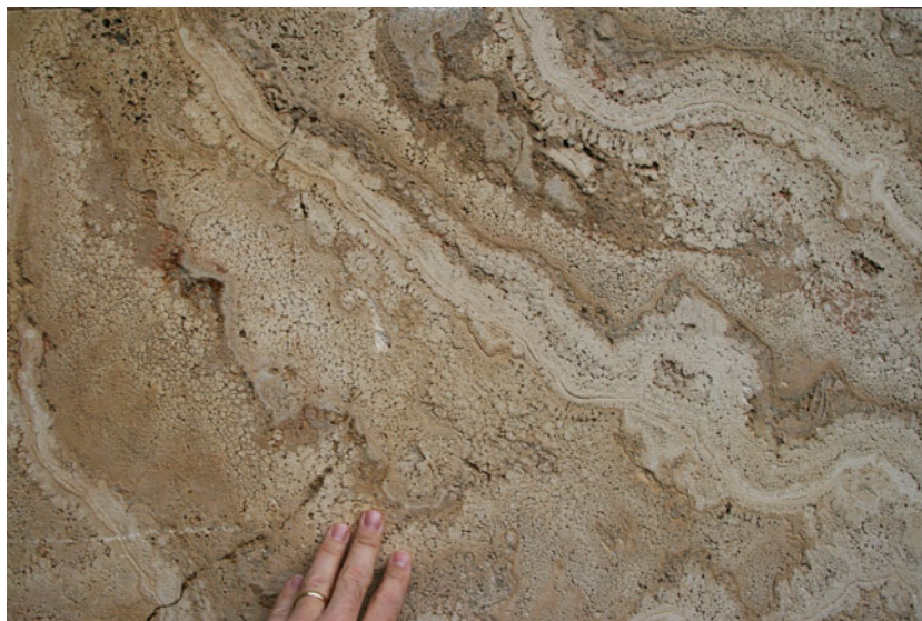
Carbonate Environments, Figure 3 Photo of sliced Quaternary tufa deposit on Casino building of Goethe University, Frankfurt, Germany, with microbial lamination and calcified remains of algal thalli.
